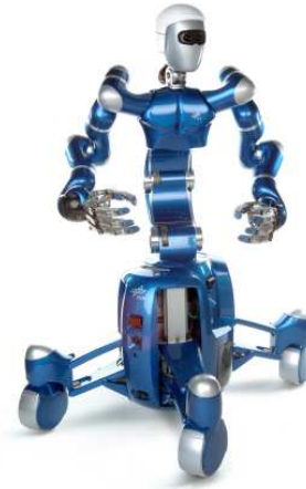
Fig. 1. DLR's humanoid Robot Justin.
