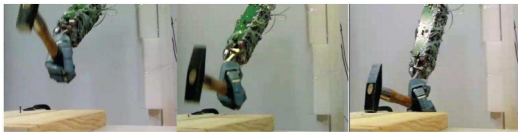
Fig. 11. Sequence of the DLR Hand Arm System driving a nail into solid wood using a 500 g standard hammer.
