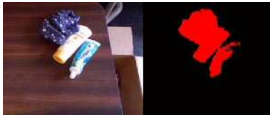
Fig. 1. Multiple objects may appear as a single segment after clustering 3D data due to lack of spatial separation.
